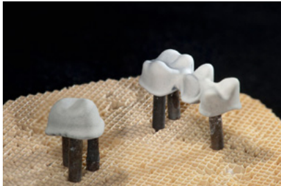
Titanium crown and bridge fixed on the firing tray after firing process
